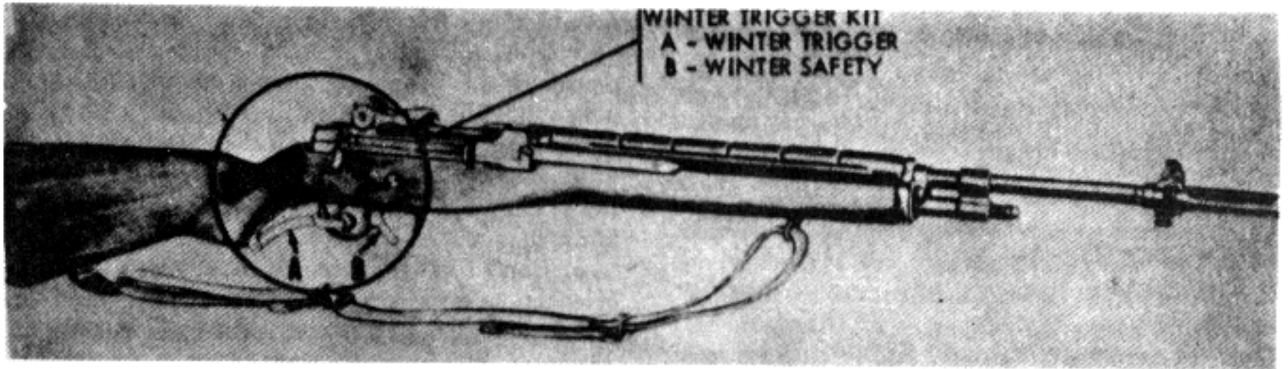
Figure 60. M14 rifle with winter trigger kit installed.
